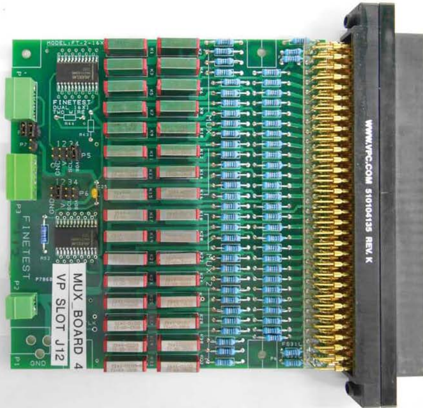
Dual 16 x 1 Mux Card with cover removed
