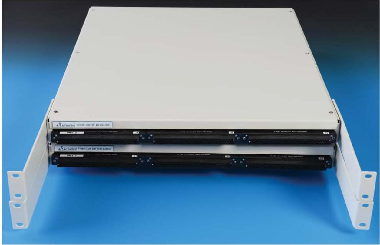
Front View of two 48x9 configured as a 96x9 Low EMF Precision Matrix
