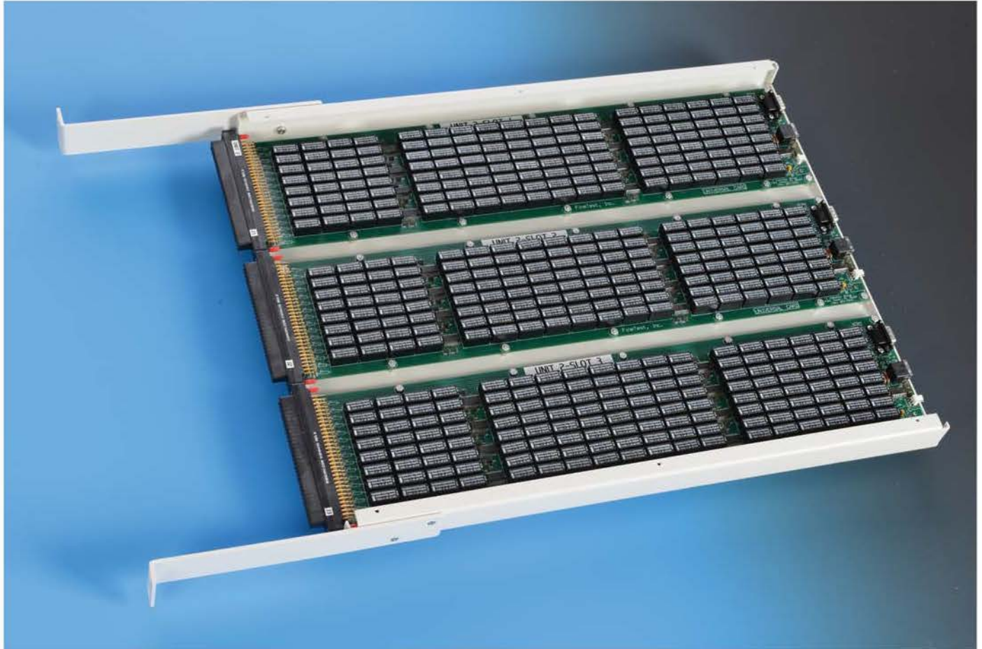
Cover removed showing 3 16x9 Cards
