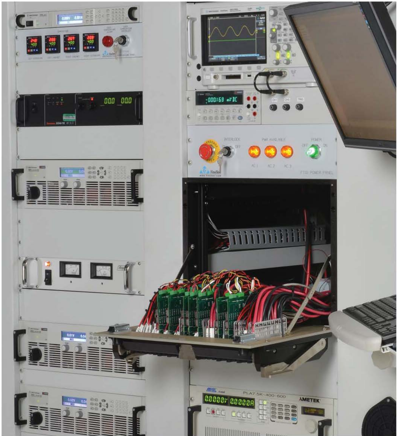
Front view of a FineTest ATE with the Virginia Panel dropped down showing multiple FineTest Switching Cards installed
