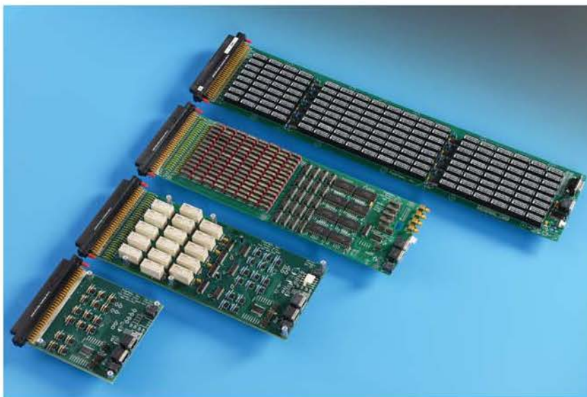
FineTest VP Cards with covers removed
