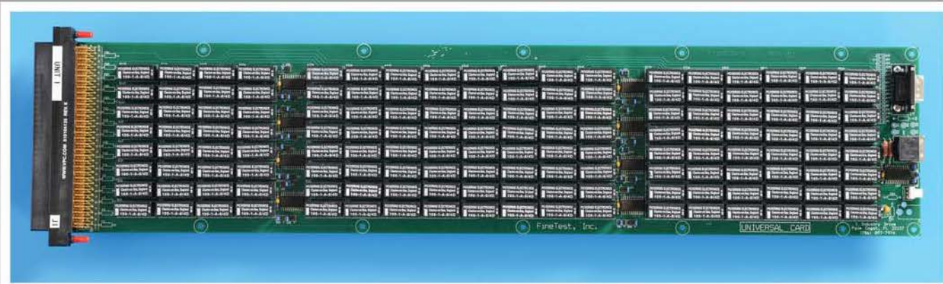
16x9 Single Wire Matrix Card with cover removed
